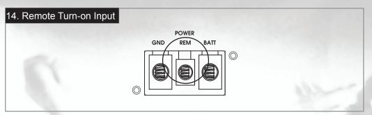
The remote terminal needs to be wired to the car's stereo or source unit remote turn on wire. This amplifier is turned on remotely when the vehicle's stereo is turned on.
